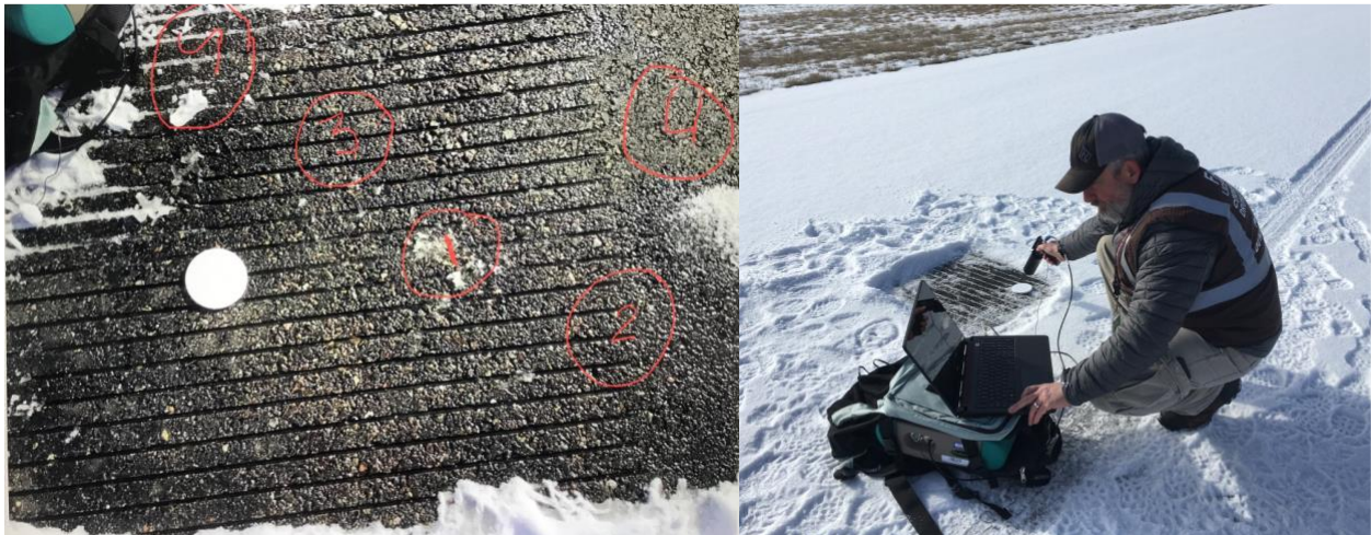
Figure 39: RGB photo of block on runway 26. Area 1 is ice, Area 2 is wet, Area 3 is wet over a grid pattern, Area 4 is dry, and Area 5 is snow. Right: data collection using spectrometer.
