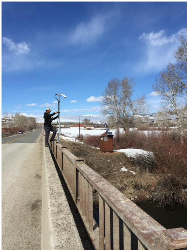
Figure 1. Photograph showing Large Scale Particle Image Velocimetry installation at the Little Blackfoot River near Garrison, Montana.
