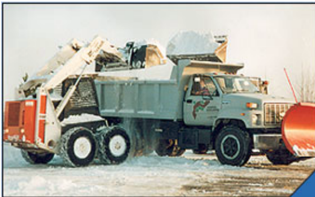
Removal of snow in sensitive areas prior to Spring melting can reduce erosion (BMP SN-1).
