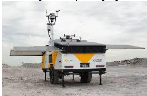
Figure 2. The Sphere Drones off-grid trailer solution (Sphere, 2025).
