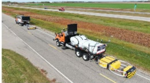
NCDOT's autonomous attenuator truck will lead a line of vehicles, which it will then follow while being monitored and controlled by an operator in a lead vehicle.
