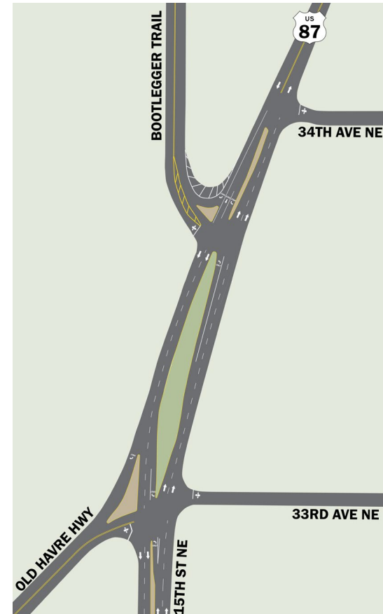
The intersection of Old Havre Highway and US 87 is complex, with unfavorable geometry.
