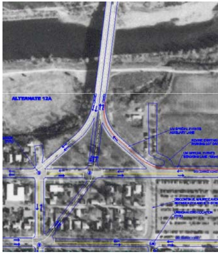
Adding a New Intersection at 5 th Street
