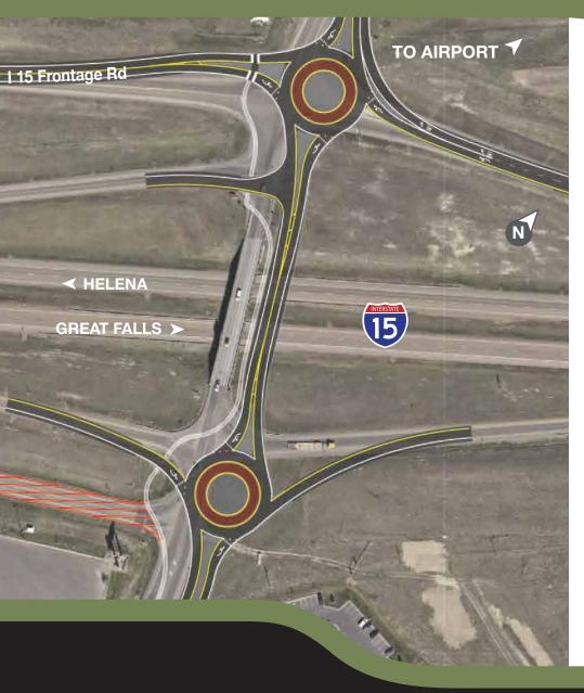
Two roundabouts are replacing the on- and off-ramp intersections. The current intersections are difficult for trucks or other commercial vehicles to navigate. This leads to reduced traffic flow.
