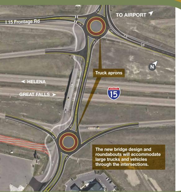
The new single-lane roundabouts will include truck aprons in the center of the roundabout.
