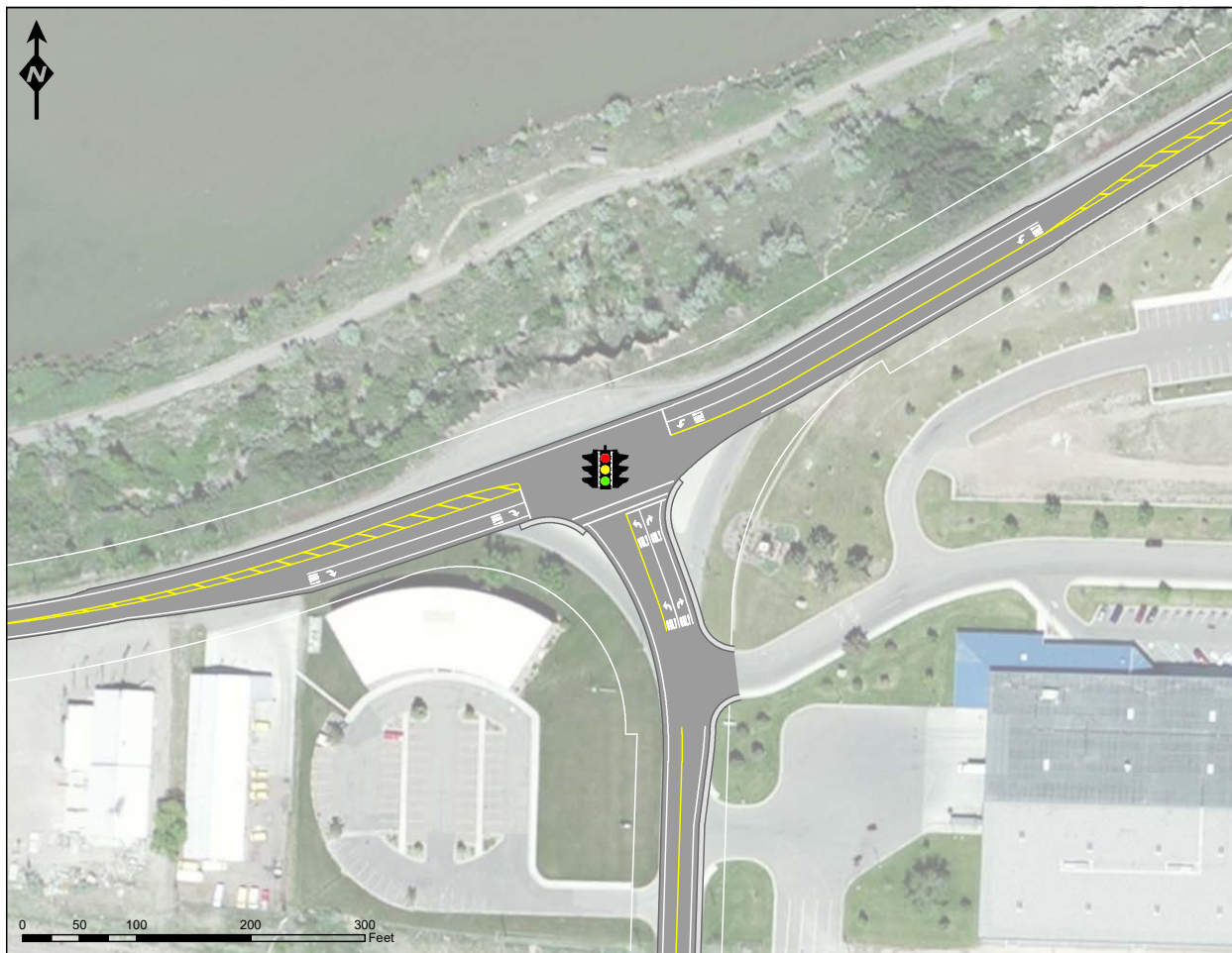
Figure 2.1: Traffic Signal Concept at 25 th Street Intersection
