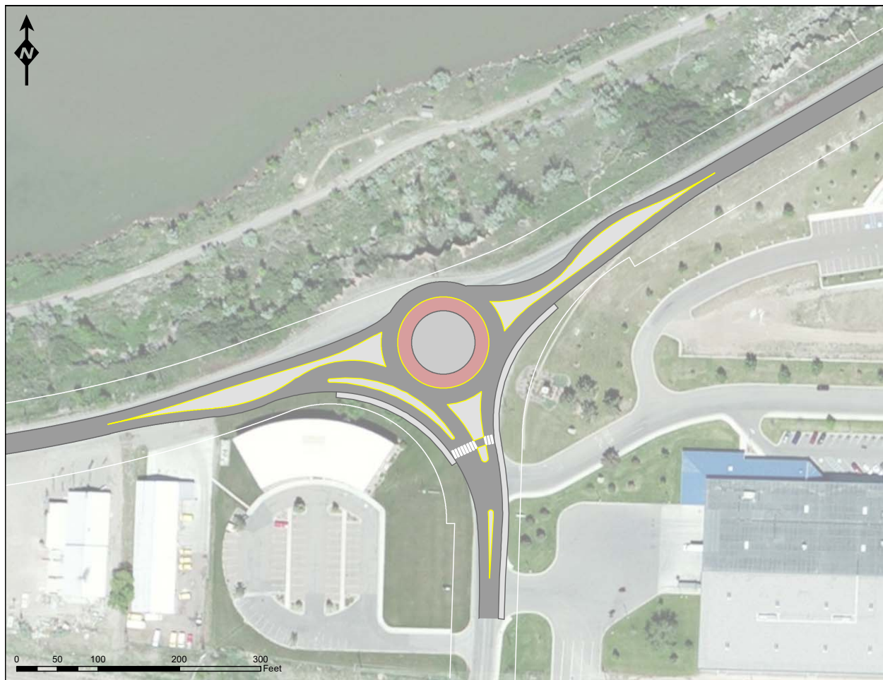
Figure 2.2: Roundabout Concept at 25 th Street Intersection
