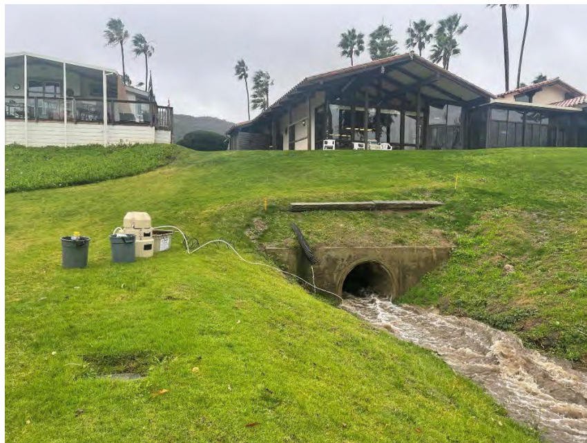
Figure 4-8a. Example of Temporary Automated Sampler Setup
