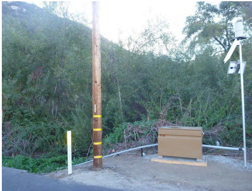
Figure 4-7. Example of Permanent Automated Sampler Enclosure
