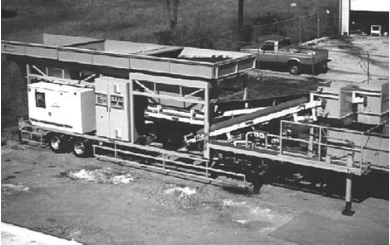
Figure 16-11: Conventional CCPR plant
