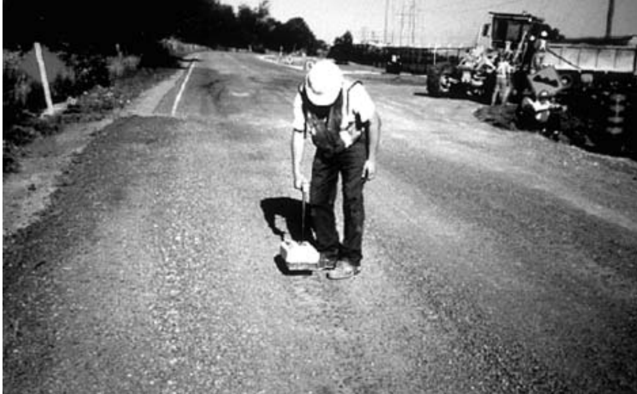
Figure 17-5: Nuclear density meter
