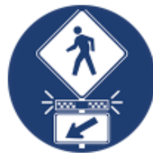
Rectangular Rapid Flashing Beacons (RRFB)
