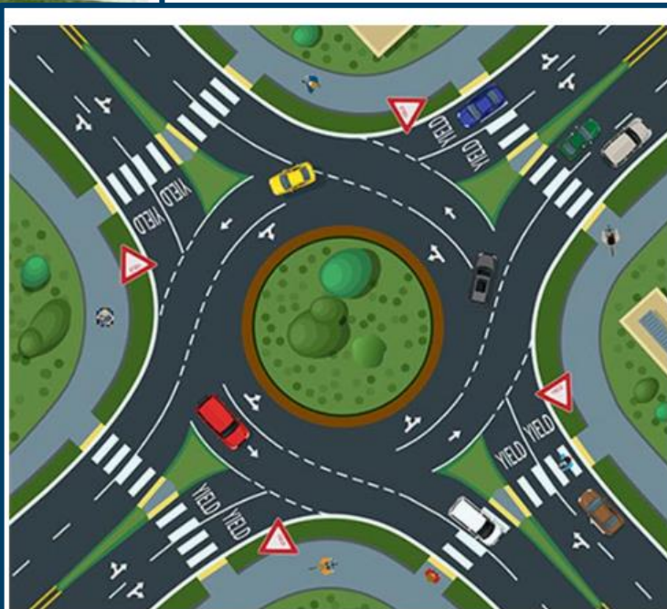
Illustration of a multi-lane roundabout. Source: FHWA
